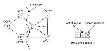
The second iteration of the while loop processes the vertex a, leading to c's discovery. The algorithm reassigns l(c) from  $+\infty$  to l(a) + 1, which is 2. Similarly, in the third iteration, l(d) is set to l(b) + 1, which is also 2:
