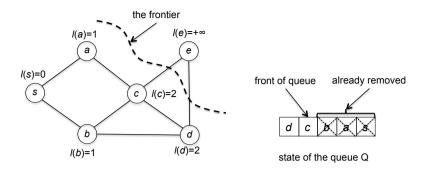
The fourth iteration discovers the final vertex e via the vertex c, and sets l(e) to l(c) + 1, which is 3. At this point, for every vertex v, l(v)equals the true shortest-path distance dist(s, v), which also equals the number of the layer that contains v (Figure 8.6). These properties hold in general, and not just for this example.
