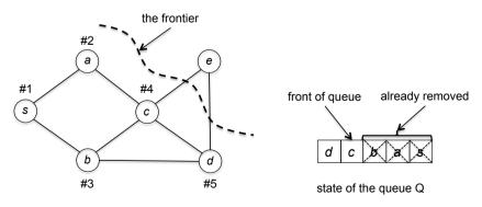
In the fourth iteration, the vertex c is removed from the front of the queue. Of its neighbors, the vertex e is the only one not encountered
