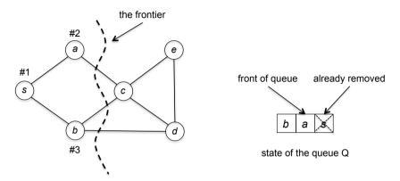
The next iteration of the while loop extracts the vertex a from the front of the queue, and considers its incident edges (s, a) and (a, c). It skips over the former after double-checking that s is already marked as explored, and adds the (previously unexplored) vertex c to the end of the queue. The third iteration extracts the vertex b from the front of the queue and adds vertex d to the end (because s and c are already marked as explored, they are skipped over). The new picture is:
