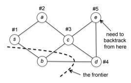
From e, DFS has nowhere to go—both of e's neighbors are already marked as explored. DFS is forced to retreat to the previous vertex, namely d, and resume exploring the rest of its neighbors. From d, DFS will discover the final vertex b (perhaps after checking c and finding it marked as explored). Once at b, the dominoes fall quickly. DFS
